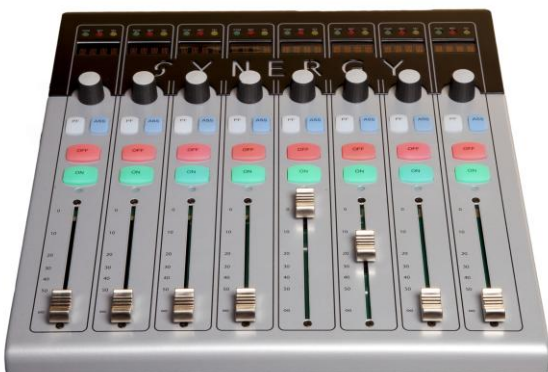
Second control surface with a further 8 fader strips, fully assignable, with unlimited user presets
